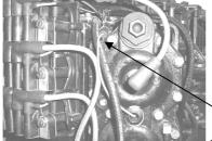
Unacceptable routing for the temp wire (V6 engine shown)
