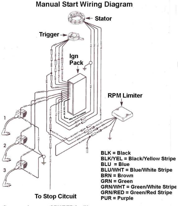
NOTE: Some engines use GRN/RED for #1, GRN/WHT for #2 and GRN for #3 cylinder. If engine backfires or seems to be out of time, index the flywheel and verify timing on each cylinder. Adjust the Green wires to reflect the correct firing order for your engine.
