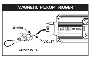
Figure 8 Checking for Spark with the Mag Pickup.
