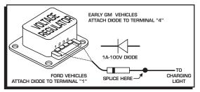
Figure 4 Installing the diode to a GM or Ford Engines.
