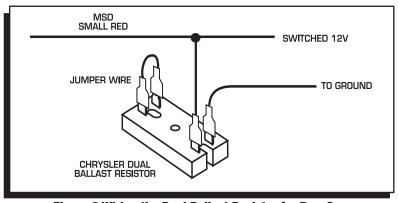
Figure 6 Wiring the Dual Ballast Resistor for Run-On.
