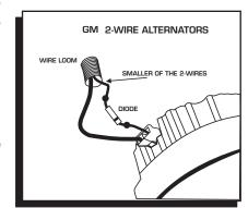
Figure 5 Installing the Diode to a 1973-1983 GM Engines.
