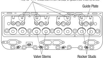
Figure 4 - Pushrod Guide Plate Clearance
