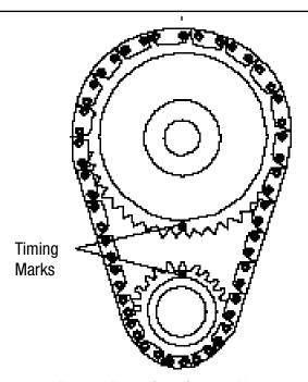
Figure 2- Timing Chain Sprocket Alignment
