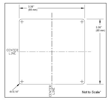
Figure 7: Mounting Template for Flush Mount Dash Installation
