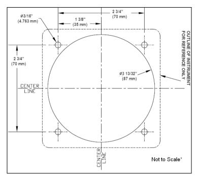
Figure 8: Mounting Template for Through the Dash Installation
