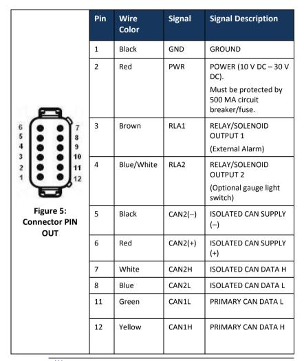
Pin 5, Pin 6, Pin 7, and Pin 8 together form a DeviceNet CAN cable. The DeviceNet CAN cable is used to receive or transmit the NMEA2000 data.
