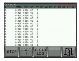
Figure 33: CAN Viewer: Recording Screen
