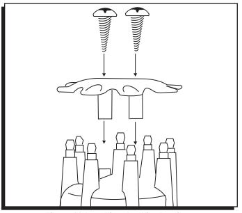
Figure 10 Installing the Wire Retainer.
