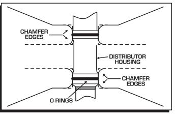
Figure 9 Modified Chevy Block for use with O-Rings.
