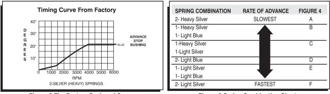
Figure 2 The Factory Equipped Curve.
