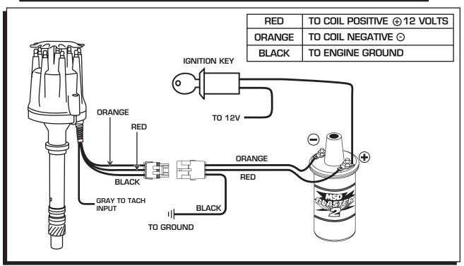
Figure 11 Wiring the Marine Ready-to-Run Distributor.
