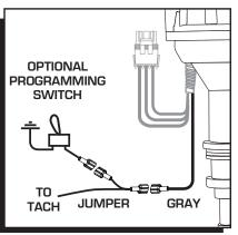
Figure 13 Setting the Rev Limiter.
