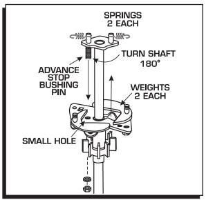
Figure 7 Locking Out the Advance.
