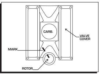
Figure 8 Marking the Rotor Location.
