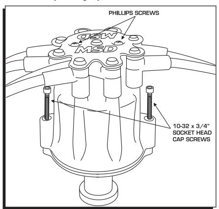
Figure 1 Installing the Wire Retainer.
