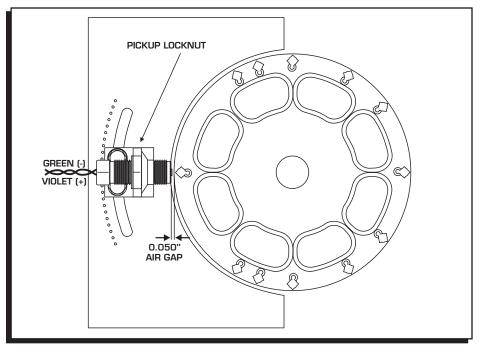
Figure 5 Setting the Pickup Air Gap.
