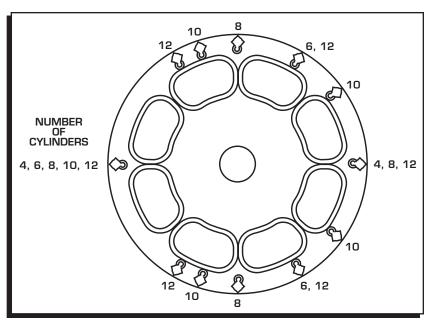
Figure 1 Magnet Location for Different Engine Applications.
