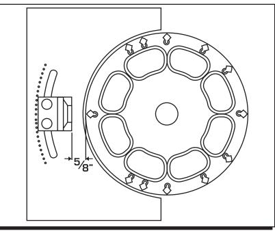
Figure 3 Pickup Bracket Placement.
