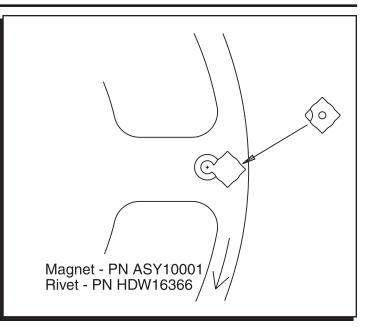
Figure 2 Installing the Magnets.
