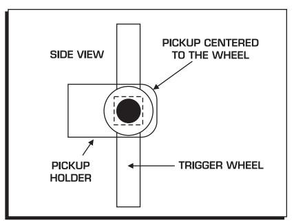
Figure 4 Centering the Pickup Mounting Hole.
