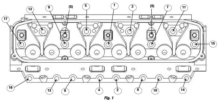
**Diagram Showing Correct Cylinder Head Tightening Sequence**
