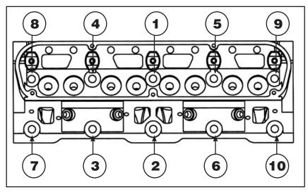
Figure 1 - Tightening Sequence
