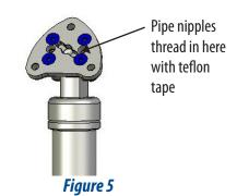
Tighten 5/16-18 x 5/8" machine screws to attach the actuator to the trim tab.
