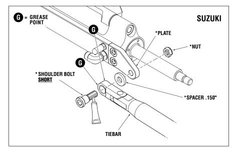
Figure 17. Suzuki Tiebar to Cylinder Installation.
