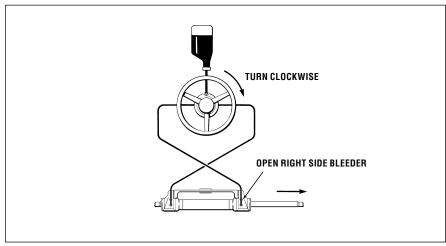
Figure 28. Tournament, Front Mount Cylinder.
