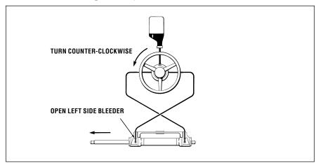
Figure 30. Tournament, Front Mount Cylinder.
