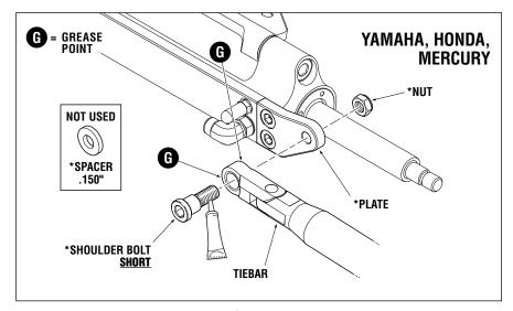
Figure 16. Yamaha, Honda, Mercury Tiebar to Cylinder Installation.
