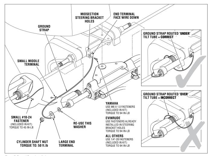
Figure 7. Ground Strap Installation.
