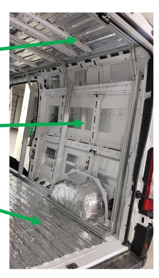
\*\* NOTE: There is no surface cleaning or degreasing required with HushMat. We do not recommend using acetone or other degreasing agents prior to installing HushMat. Simply wipe our any dust or dirt using a lightly dampened cloth, allow to air dry and then install HushMat. HushMat absorbs surface oils on the van and uses them as an adhesion promotor.
