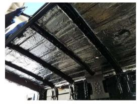
We used installation photos from a Black Van using our HushMat Silver sound deadening & thermal insulation material for this roof installation
