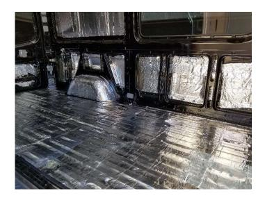
HushMat sound deadening & thermal insulation material floor, sidewalls, rear doors and roof - installed.
